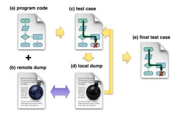
Figure 3. How RECORE works. Given a executable program (a) and a remote core dump (b), RECORE generates tests (c) whose final state (d) is then compared to the original core dump (b). The test generator systematically evolves the test case to increase similarity. The final test case (e) makes the program fail with the exact same stack trace.
